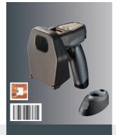
Mobile combination device with Bluetooth Bar code/RFID HF (13.56 MHz) Transponder: ISO 15693 Bar codes: Code 39; Code 128; Code 93; EAN 8/13; 2/5 Int. (all common) 0-30mm 0-450mm no RS 232 via 9-pin Sub-D USB converter cable 230V AC (3.7V DC batt.) 200 mA IP 54 (base: IP 54) 1m (base: 1m)
