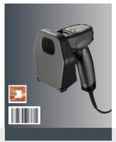
Mobile combination device Bar code/RFID HF (13.56 MHz) Transponder: ISO 15693 Bar codes: Code 39; Code 128; Code 93; EAN 8/13; 2/5 Int. (all common) 0-30mm П 0-450mm no RS 232 via 9-pin Sub-D USB converter cable 5V DC
