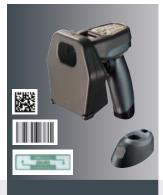
Mobile combination device with Bluetooth 2D/Bar code/RFID UHF (868/915 MHz) Transponder: EPC 1 Gen 2 Bar codes: Code 39; Code 128; Code 93; EAN 8/13; 2/5 Int. (all common) 2D-codes: ECC 200; PDF 417: GS1 Databar 0-450mm 30-350mm 10-150mm RS 232 via 9-pin Sub-D USB converter cable 230 V AC (3.7 V DC batt.) 200 mA IP 54 (base: IP 54) 1m (base: 1m) 380g (base: 200g)
